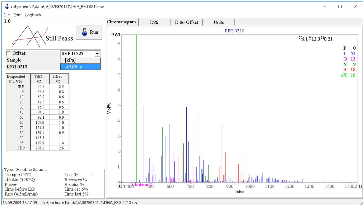
The sample has been recognized as Summer Spec gasoline and the ASTM D86 cross check data are displayed at the left side. The setpoints and offsets for this summer gasoline are found in the D 86 Offset tabsheet:
