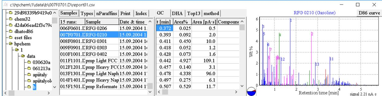
The white slice of the small circle at the left bottom of the chromatogram indicates almost 50% of the sample peaks are not identified.
