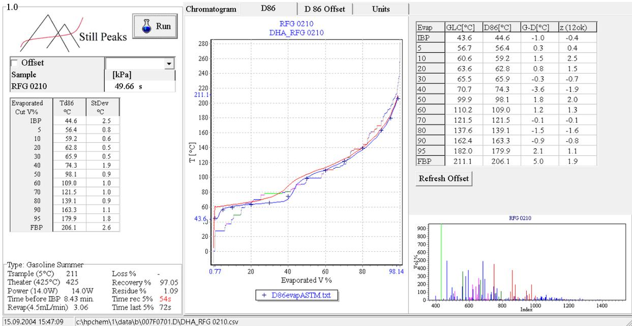
Next we change the Delay setpoint and the Eo number in a last effort to get closer to the ASTM D 86 data:
