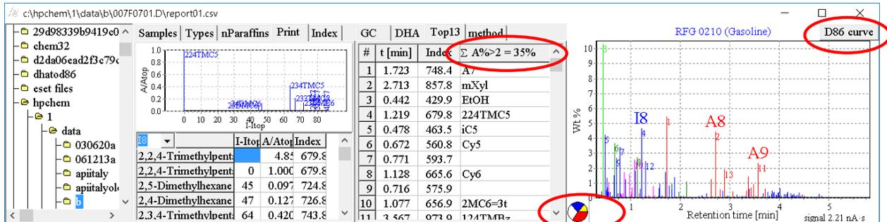
The left hand tab sheet Print is selected, where the hard coded I8 pattern is selected. This pattern is recognized in this sample and marked with I8. The yellow part of the ID pie indicates that about 20% of the peaks in this sample are identified by peak recognition of the Iso-octanes (I8), Xylenes and Ethylbenzene (A8, A9).
