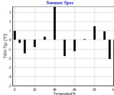
The offset values are the negative values of the G-D data column in above D86 report. When we recalculate using these offsets we get:
