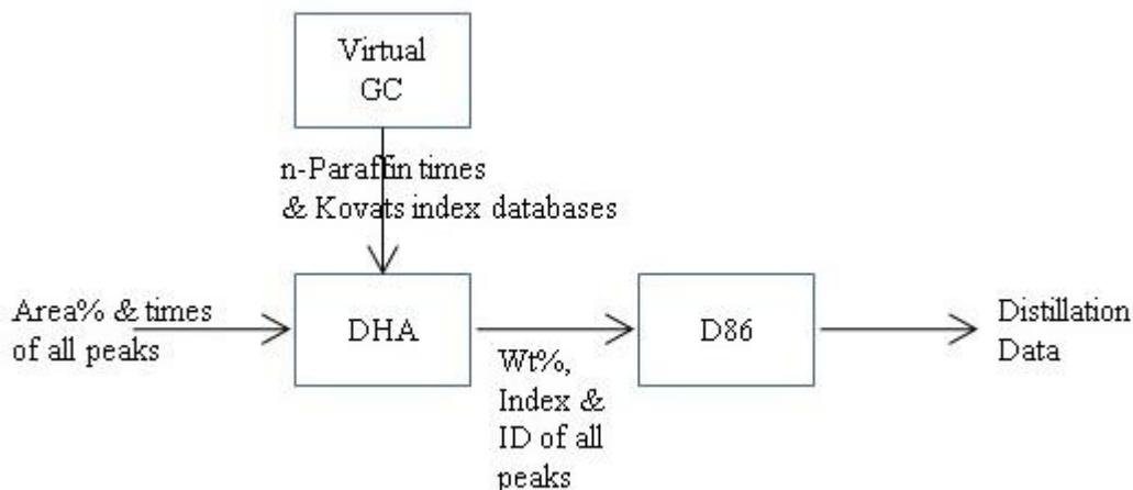
**Virtual GC** is a computer model of a Dimethylsilicone coated capillary gas chromatographic column. Kovats index databases and n-Paraffin retention times are calculated from GC configuration input and an isothermal Kovats index database. The GC configuration should match the actual GC configuration. Column aging is accounted for with film thickness. Copy the Virtual GC window to your lab journal.
