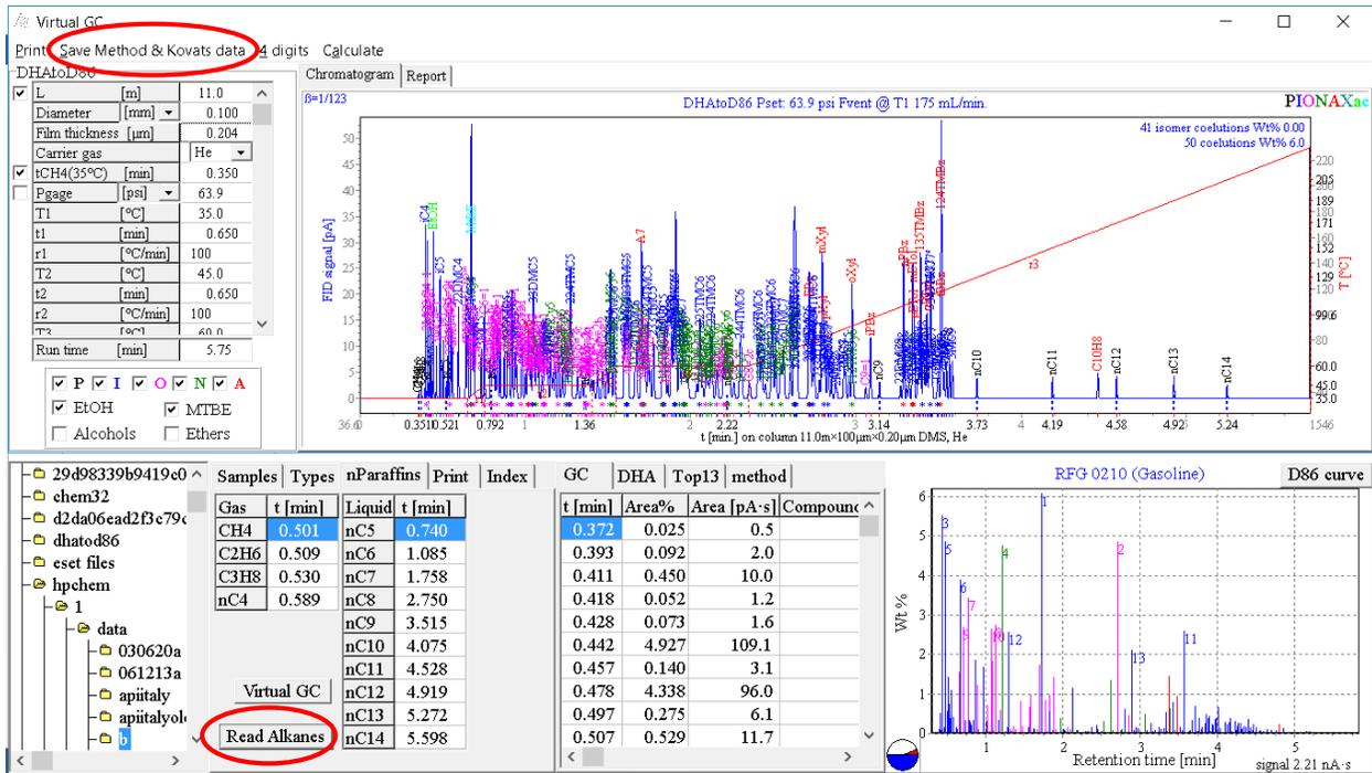
Select the Save Method & Kovats index data menu option of Virtual GC. Times and databases are filed. Select the Print option of the Virtual GC menu to keep track of the n-Paraffin calculations. The n-Paraffin times and databases are applied in DHA only after clicking the Read Alkanes button:
